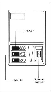
NOTE: at high volume settings, audio feedback from microphone may cause a squealing sound. Lower the volume level to eliminate this sound.
